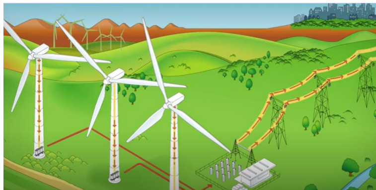
Diagram: The Process of Electricity Generated by Wind Power Plants
